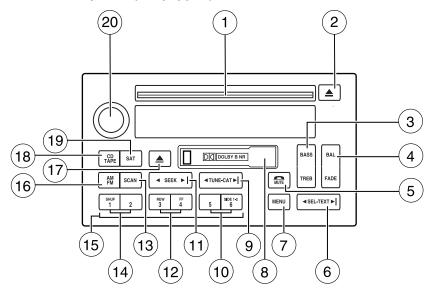
1. **CD slot:** Insert a CD, label side up. With the ignition on, the radio will begin to play a CD once
